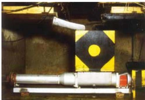
A custom-built W082 is speeding up waste disposal at a Scottish tannery. Previously the 'fleshings' were shovelled manually from the processing area to a skip, this method was highly labour intensive. The cast iron W range pump with large auger and hopper were specially modified in order to handle this difficult material. The fleshings waste is gravity fed into the hopper, then pumped at 5.5m<sup>3</sup>/h at a pressure of 3 bar, along 30m of pipe direct to an outside skip for disposal.
