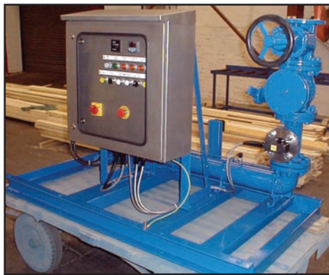
Skid mounted package comprising pump, gearbox, control panel, baseplate and suction and delivery pipework connections
