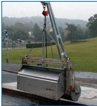
Lifting chain management system for a Mono Stormscreen
