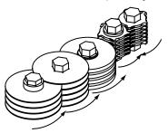
Path of solids being transported across the face of the screen directly into the cutters.
