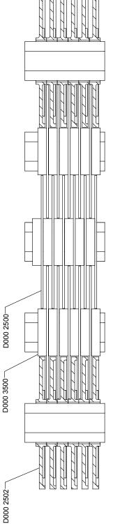
9mm (0.35") DISCREEN DISC AND SPACER BUILD 5 SHAFT CONFIGURATION EXAMPLE D000 2502 DISCS ARE ASSEMBLED ON THE OUTER SHAFTS OF ALL ASSEMBLY CONFIGURATIONS TO MAINTAIN REQUIRED SCREEN APERTURE. NB. D000 2502 DISCS ARE SECTIONED FOR CLARITY.
