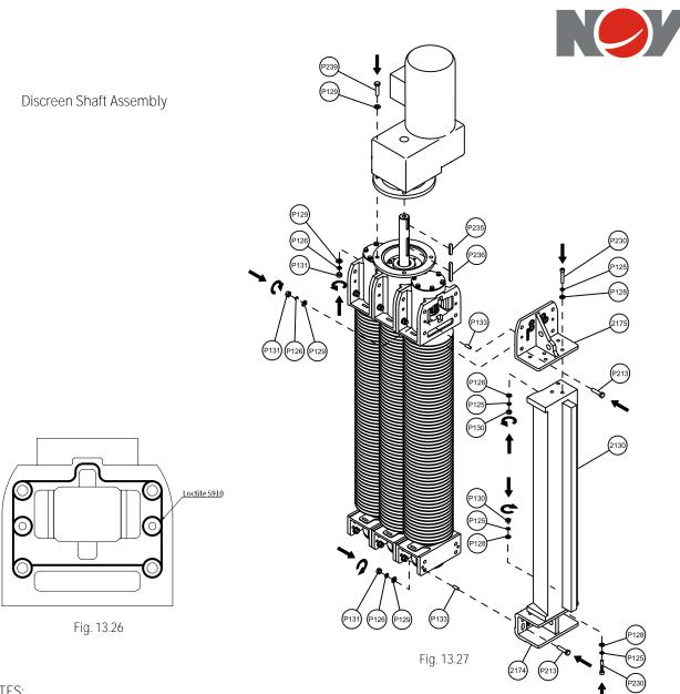
• Seal the faces between the top housing and top mounting bracket (2175) using Loctite 5910 see Fig. 13.26
