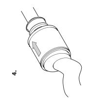
MUST BE FILLED WITH OIL IN THE VERTICAL POSITION
