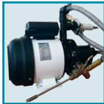
Brine Injection Unit
